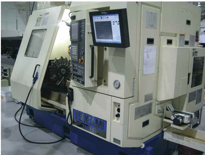
The new Tsugami TMU1 Swiss Mill/Turn machine capable of 1-1/2" diameter turning.
